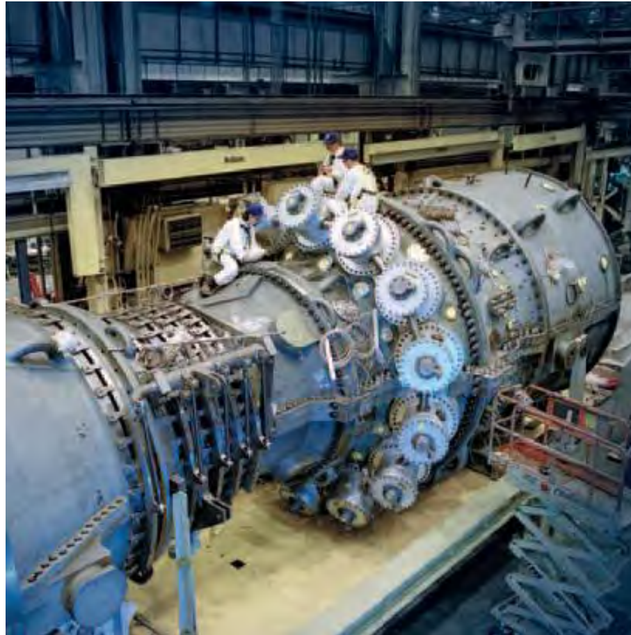
Combustors on a GE 7H gas turbine.
